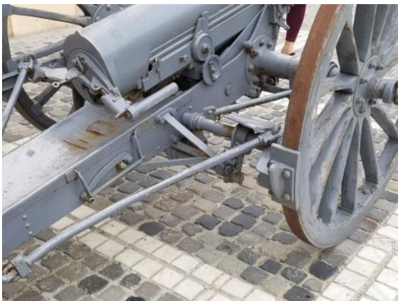
Here's the right side of a gun located at the old town square in Brazov, Romania. Note again the placement of the tie rods.
